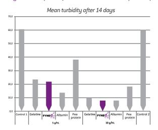
Turbidity analysis (in NTU) after fining for 14 days at ambient temperature in a laboratory.
