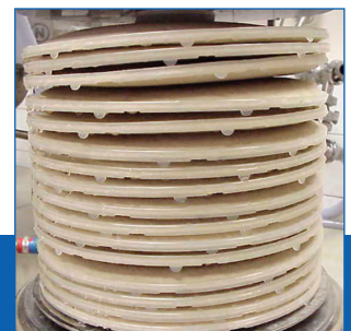
Cell deformities after heat treatment
