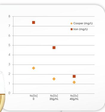
The chelating effect of fungal polysaccharides eliminates copper and iron, specific catalysts of all oxidation processes. The test below assessed the yellow tint (OD420nm) of a white wine. It demonstrates the indisputable curative action of No[0x]on the colour of oxidised wine.
